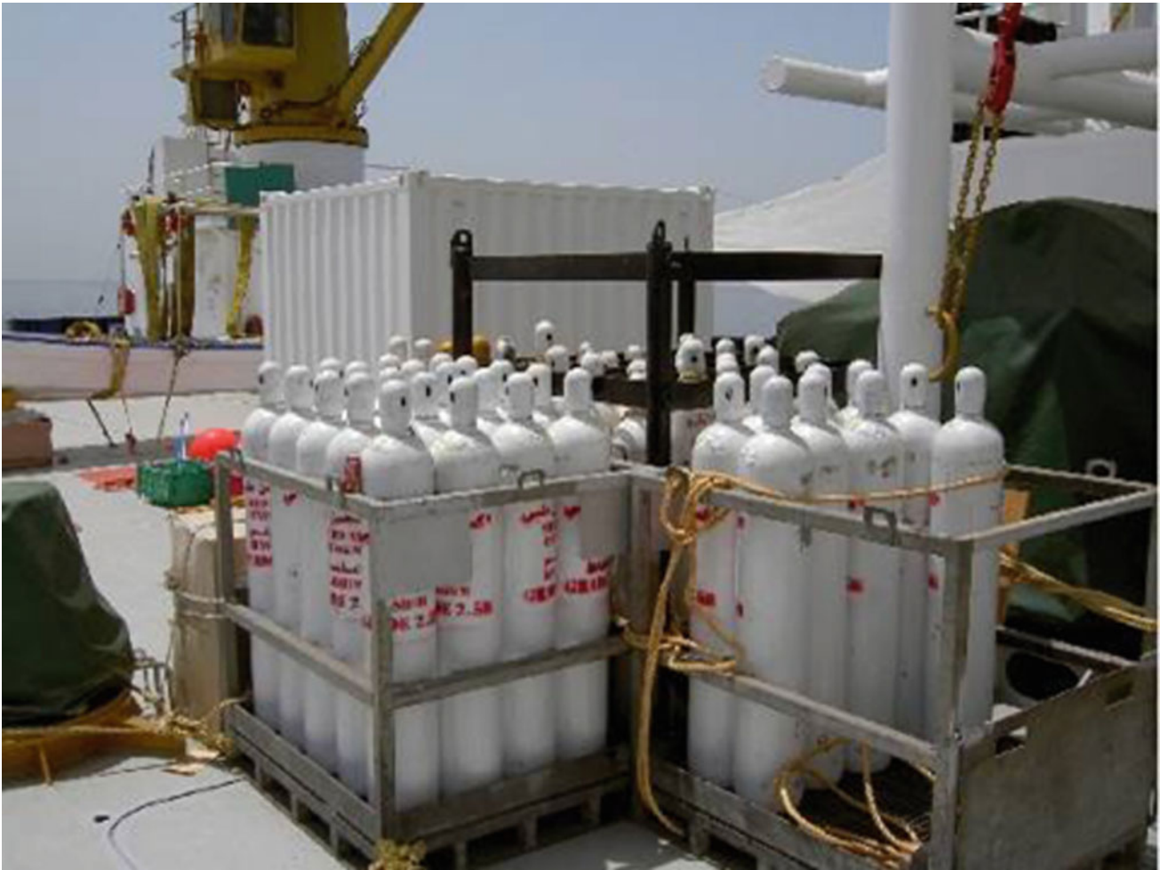
Fig. 4 Pure oxygen on the back deck of the MV Midyan to be mixed with helium and air to form Nitrox (Photo: Garry Momber)
